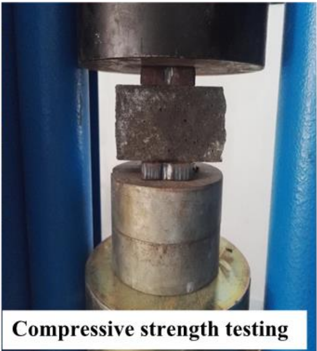
Figure 11. State of samples before testing and experimental setups of the UPV and compressive strength tests.
