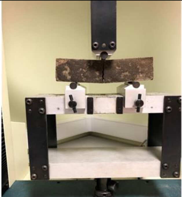
Breaking the prism into halves
