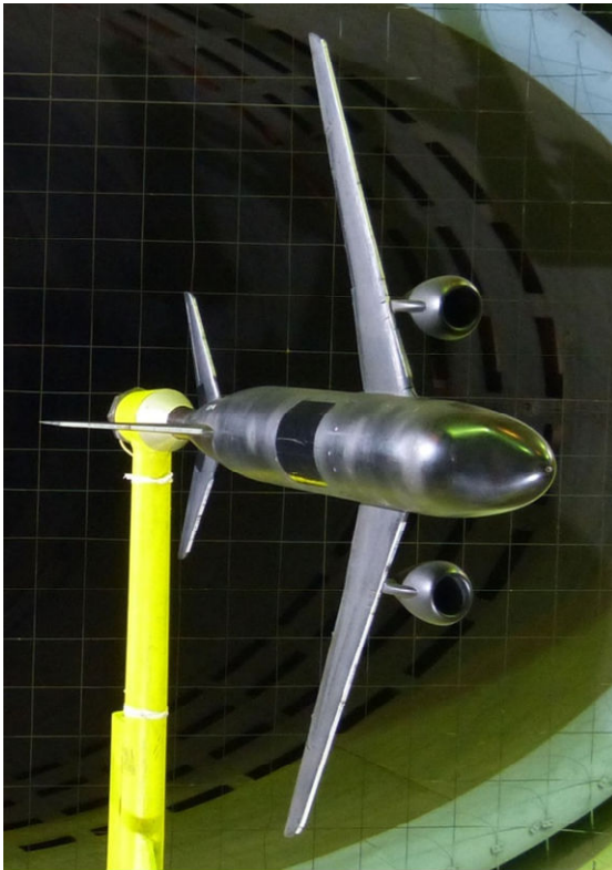
Fig.1. Fully iced aircraft model installed on the tail support strut in the wind tunnel test section.
