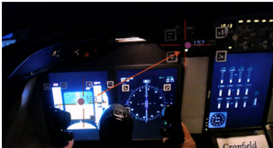
Figure 2. Pilot’s attention shifts from Primary Flight Display (fixation-156) to Flight Mode Annunciator (fixation-157) due to mode changes recorded by eye tracker
