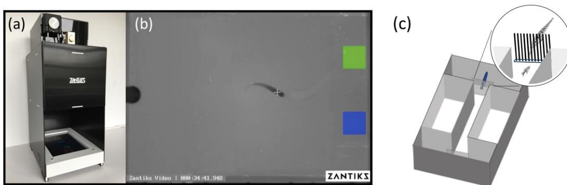
Figure 1. Experimental apparatus. (a) Lateral view of the operant conditioning chamber (Zantiks AD). Stimuli were presented using a screen positioned on the base of the tank. A camera mounted above the tank automatically detected the behaviour of the subject and sent information to a computer through a wireless internet connection. (b) Example of the experimental setting used in the operant conditioning chamber. As soon as the focal fish triggered the beginning of a trial by selecting an initiator light presented on one side of the tank (e.g., left), two squares differing in colour (e.g., green and blue) were presented on the opposite side (right). A correct choice triggered a motor to release food at the opposite end of the tank. (c) Apparatus used to test brain lateralization. The central runway allowed the fish to face a barrier. A dummy predator was visible behind the barrier at the both ends of the runway.
