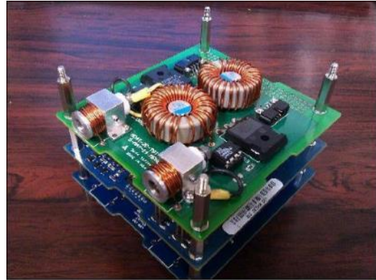
Figure 2.4 The VAT ( \mu CAT) developed by the Micro-propulsion and Nanotechnology Laboratory at the George Washington University, United States (source: https://directory.eoportal.org/web/eoportal/satellite-missions/b/bricsat-p )
