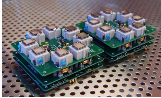
Figure 2.2 An EPT (iEPS) system developed in the Space Propulsion Laboratory at Massachusetts Institute of Technology (MIT), United States, United States (source: http://spl.mit.edu/electrospray-thruster-engineering )
