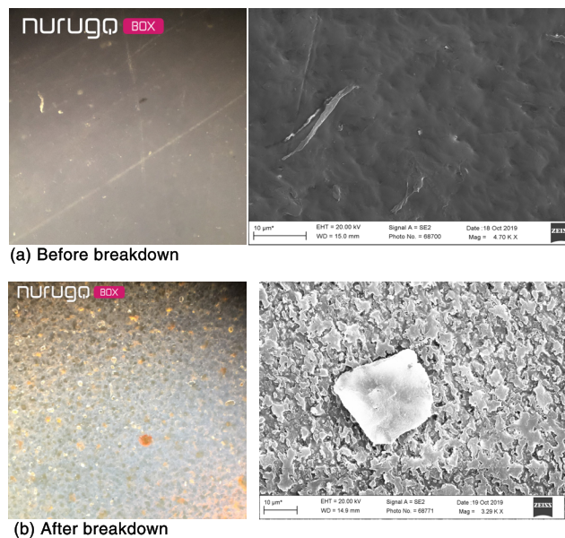
FIGURE 4. Agglomeration of nano-clay flakes separated from matrix after thermal breakdown.
