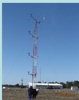
Figure 1: Picture of 10 m tower used in CIBA. 5 levels: cup anemometers, vanes and thermometers; at 1.5m and 10 m height humidity and sonic anemometers. Terrain is very flat without obstacles nearly.
