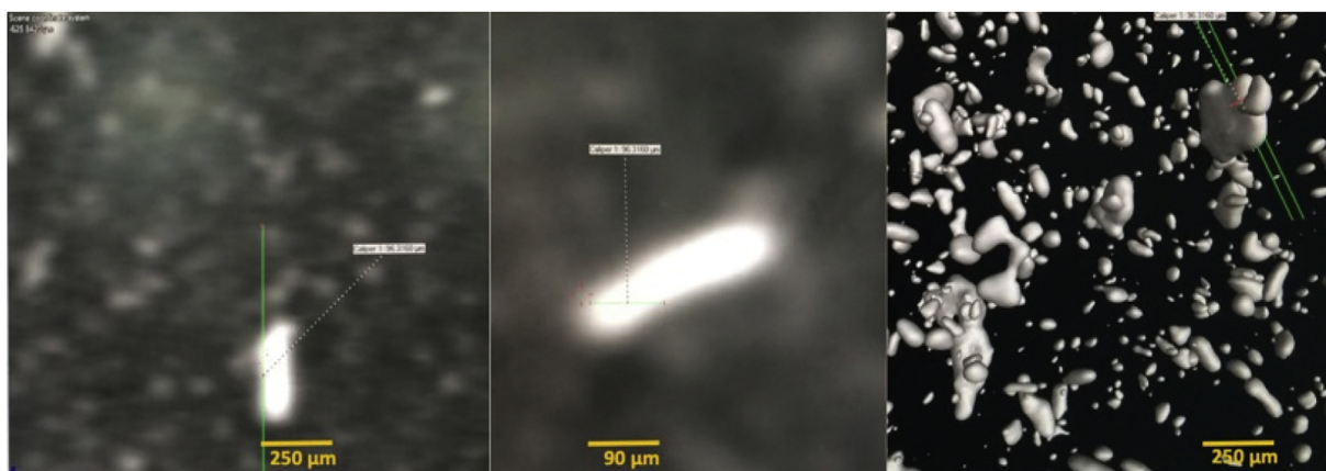
Fig. 5. X-ray CT of sintered calcium aluminate material with Ag.
