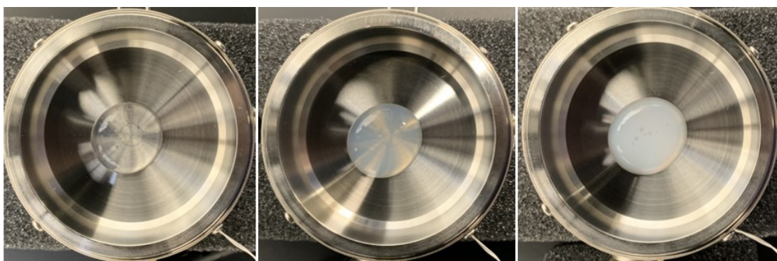
Figure 11. A 30.0% (w/w) Soluplus ® solution at room temperature (left), cloud point (middle) and gel point (right). Represented as a top view of the cone-and-plate rheometer sample compartment that was lowered from its housing and subjected to increasing temperatures.
