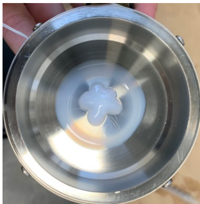
Figure 28. A gelled 20.0% (w/w) Soluplus ® solution on the plate of a cone-and-plate rheometer. The star-like shape is caused by the pulling away of the CP52 spindle when the solution is gelled. The remaining solution seen circulating around the star-like shape is where the spindle didn't come in contact the plate due to its small diameter.
