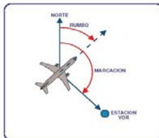
Imagen 8. V.O.R (VHF - Very High Frequency Omnidirectional Range)
