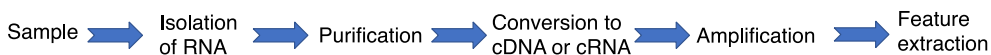
Figure 1. Workflow of a gene expression microarray experiment. RNA is isolated from our cells of interest. It is then purified, amplified, and converted to cDNA (reverse transcription) or cRNA and then loaded onto the array. Probes on the array are then hybridized and signal intensities of the features are obtained after scanning.
