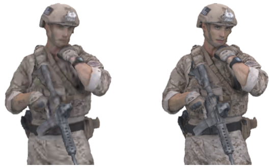
Fig. 2: Two representations of the soldier object: R1 at 4.5 Mb/s (left) and R5 at 40.4 Mb/s (right).
