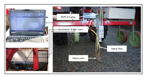
**Figure 2.** The on-line visible and near infrared (vis-NIR) spectroscopy sensor developed by Mouazen [37], showing the main components (**right**) and the on-line spectral data acquisition (**left**).
