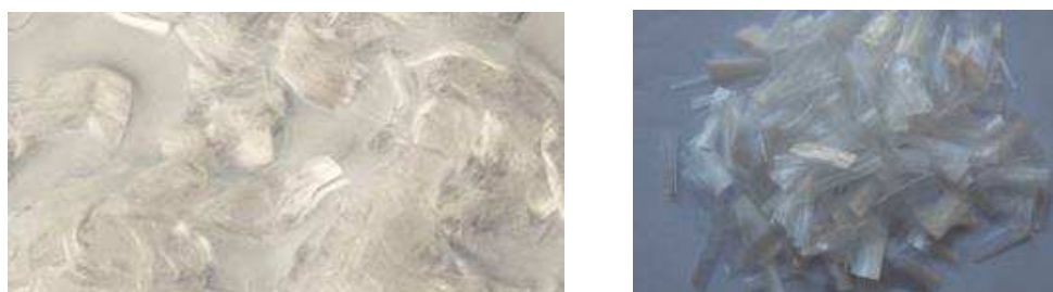
Figure 2 Polypropylene (PP) fibres: a): RoWhite (PP1); b) al ECONO NET (PP2)
