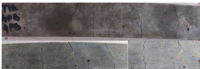
Figure 9 SS-L mix, 4PB multiple cracking: a) initial; b), c) crack closing after curing exposure
