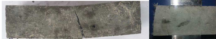
Figure 5 Mixture SS-L: Failure and cracking pattern under tension and compression
