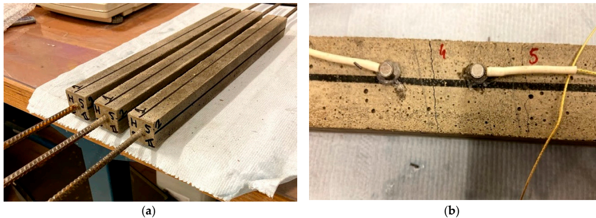
Figure 4. Specimens used during wet-dry healing cycles: (a) geometry of the specimens with central rebar and (b) positioning of the sensors around the crack opening.
