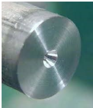
Figure 15: Tail-Stock center hole
