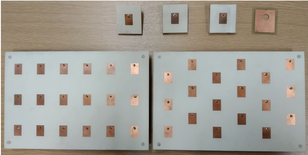
Fig. 4: Front views of the fabricated single antenna and antenna arrays. The ground plane of the antenna is presented in the top-right corner.
