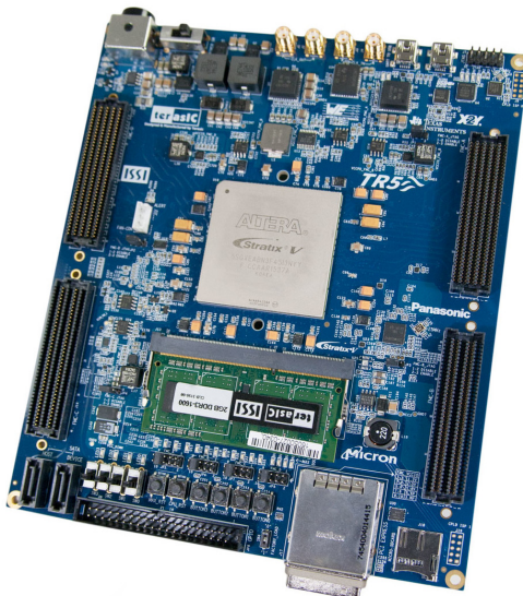
Figure 2.2: Terasic TR5 development kit
