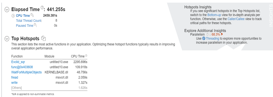
Fig. 2.30: Execution time of the Kohonen neural network training for all digits using OpenMP
