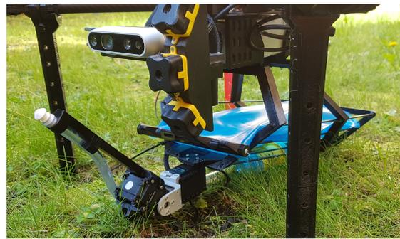
(b) Mounted fire extinguisher detail
