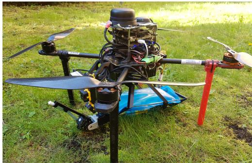
(a) UAV with mounted fire extinguisher
