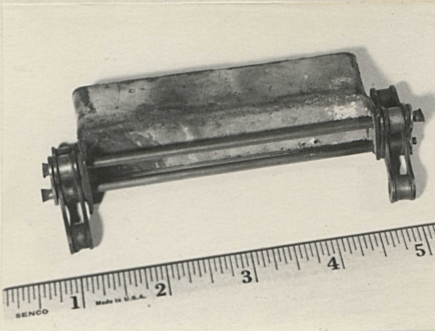
Photo showing scraper attachment to chain.
