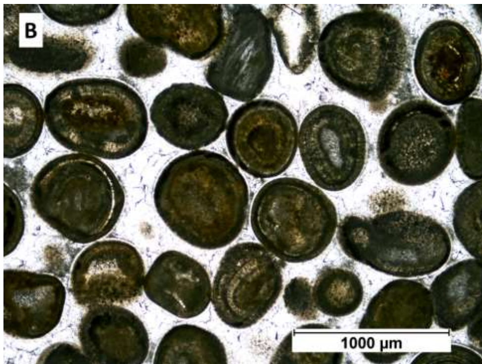
Figure 3. Bath Stone in thin-section. B: Bath Oolite: dominated by ooids, with a calcite spar cement. Thin-sections prepared by Ron Smith. Brown's Folly, near Bathford.
