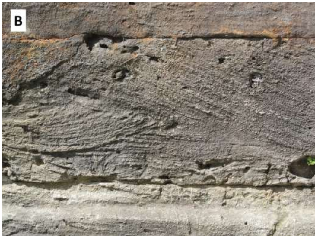
Figure 4. B: Cross-bedded shelly oolitic grainstone with burrows and cavities, a stone from the base of a Roman column. Field of view 40 x 25 cm.
