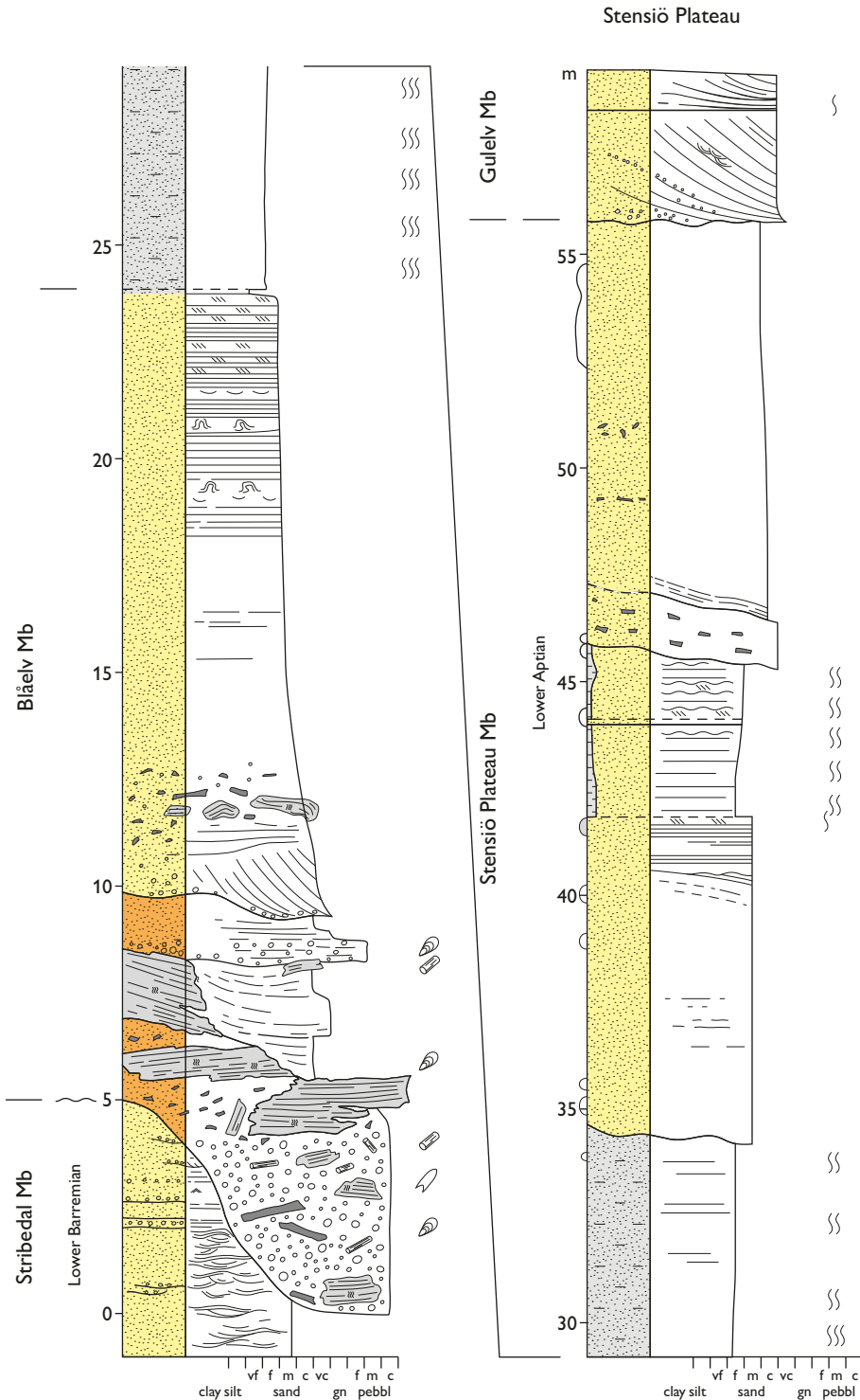
Fig. 22. Reference section of the Steensby Bjerg Formation showing gravity flow conglomerates and sandstones of the Bläelv Member and prodelta and gravity flow sandstones of the Stensiö Plateau Member at Stensiö Plateau, Hold with Hope.
