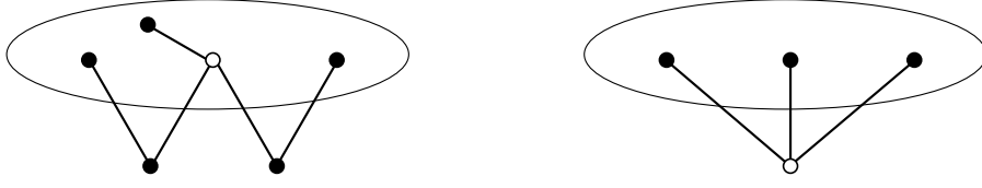
■ Figure 3 A pair of compatible configurations at a forget node. The figure on the left is the original tree, and the white vertex is the vertex being forgotten. The figure on the right is the result of the contraction.
