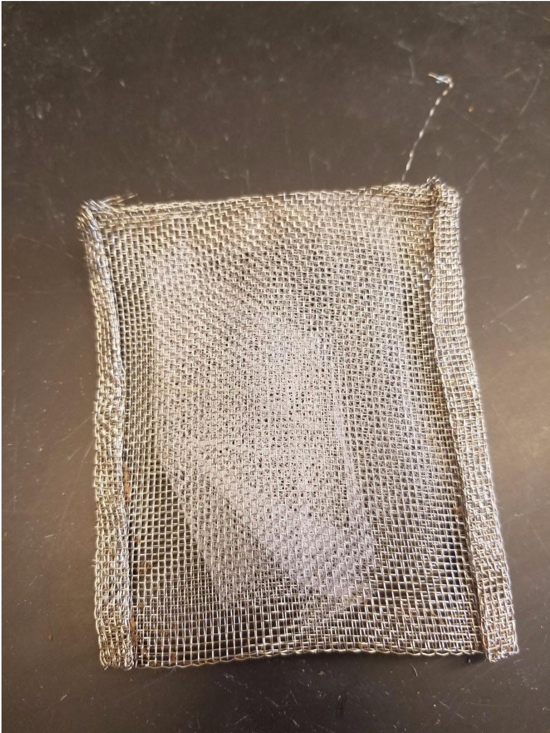
Appendix B2. A 2X3 inch seed germination packet made from nylon fabric within a stainless steel sleeve.
