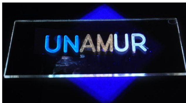
Figure 4.23. Film of the acronym of the University of Namur designed employing the trans -O-POSS (first two letters on the right), Eu@ trans -O-POSS (letters in the middle) and cis -O-POSS (last two letters on the right) under UV lamp (356 nm).
