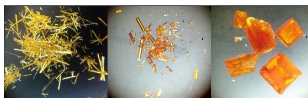
Figure 4. Single crystals of compounds 1 2 ·2F4 (left), 2 2 ·I2F4 (middle) and 3 2 ·I2F4 (right), obtained by recrystallization from solution of the mechanosynthesis products (see Experimental).
