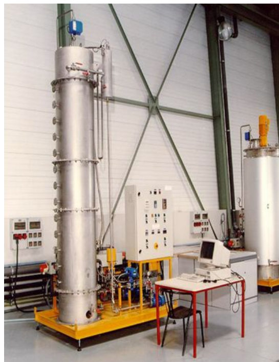
Fig. 1.3 – Anaerobic digestion pilot reactor of INRA - LBE, Narbonne, see (Gouzé and Steyer, 2007).
