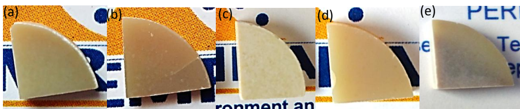
Figure 4.46. Images of samples from deagglomerated powder after annealing at 800°C-6h (see Table 4.3. for the legend). (Thickness ~ 2 mm).
