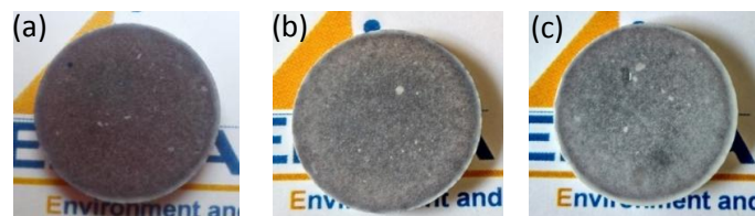
Figure 4.22. Pictures of BT samples sintered at 1000°C by SPS at heating rates of (a) 10°C/min; (b) 50°C/min and (c) 100°C/min.
