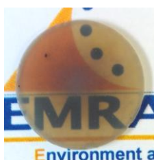
Figure 3.19. Sample sintered at 1300°C after annealing at 1100°C 24h.
