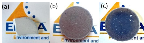
Figure 4. 19. Pictures of BT samples sintered at 1000°C by SPS at pressures of (a) 30 MPa, (b) 50 MPa and (c) 70 MPa.
