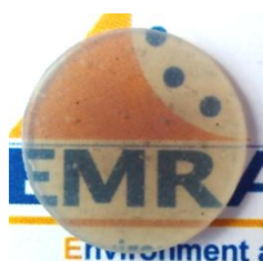
Figure 3.20. YAG-S sample sintered by SPS at 1300°C and post-treated by HIP at 1250°C for 1 h.
