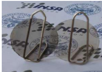
Figure 1.19. YAG samples after SPS (15 min, 1350 °C, 74 MPa) before annealing (left), and after air annealing at 800°C for 1h (right) [11].
