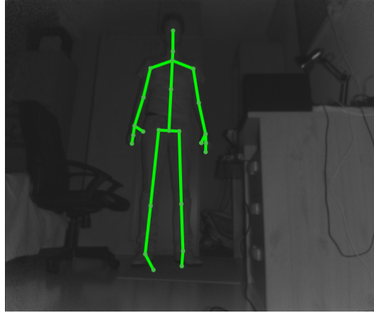
Figure 3.9: Representation of the infrared frame source.
