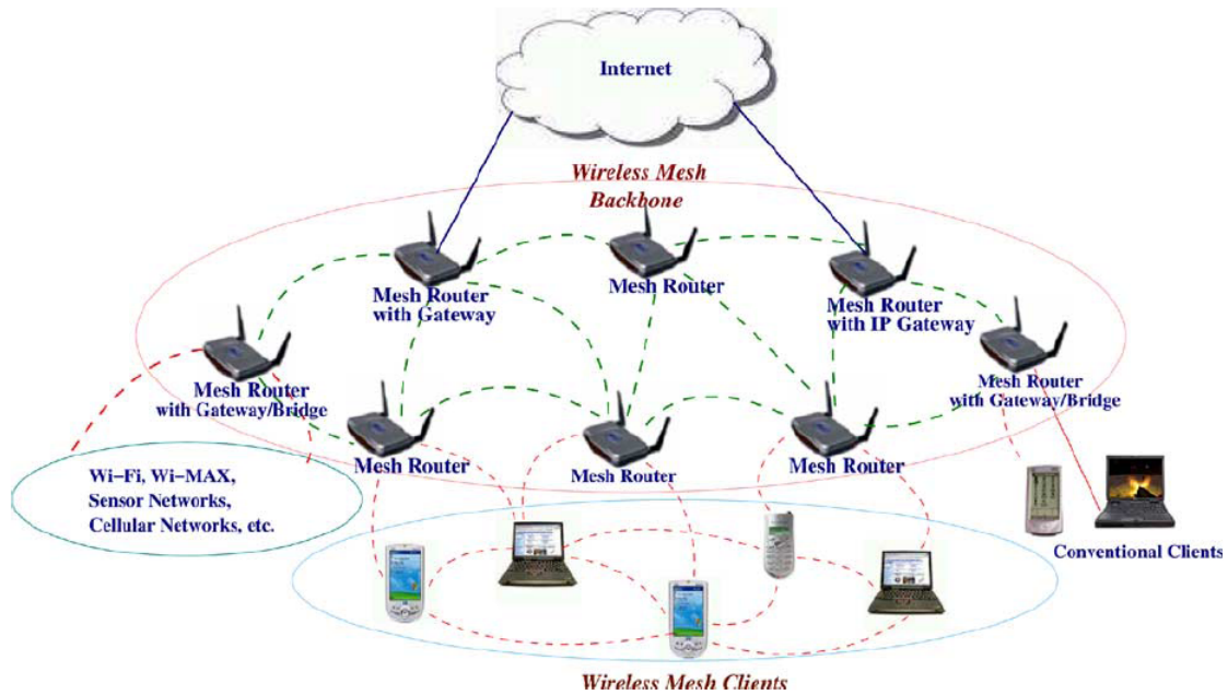
Figure 7.3: Hybrid wireless mesh network [JS]
