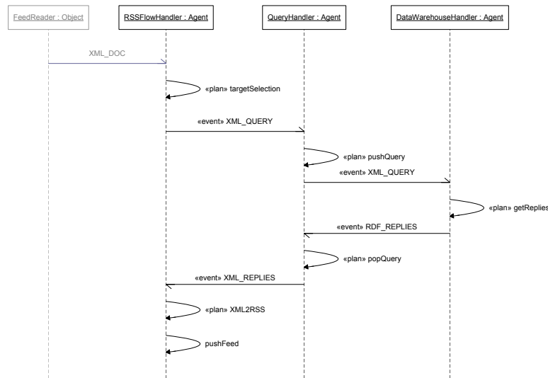
Figure 6.6 • Sequence diagram depicting the query process
