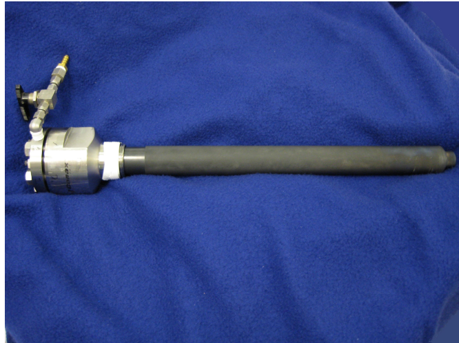
Fig.8. SiC temperature probe shown assembled.
