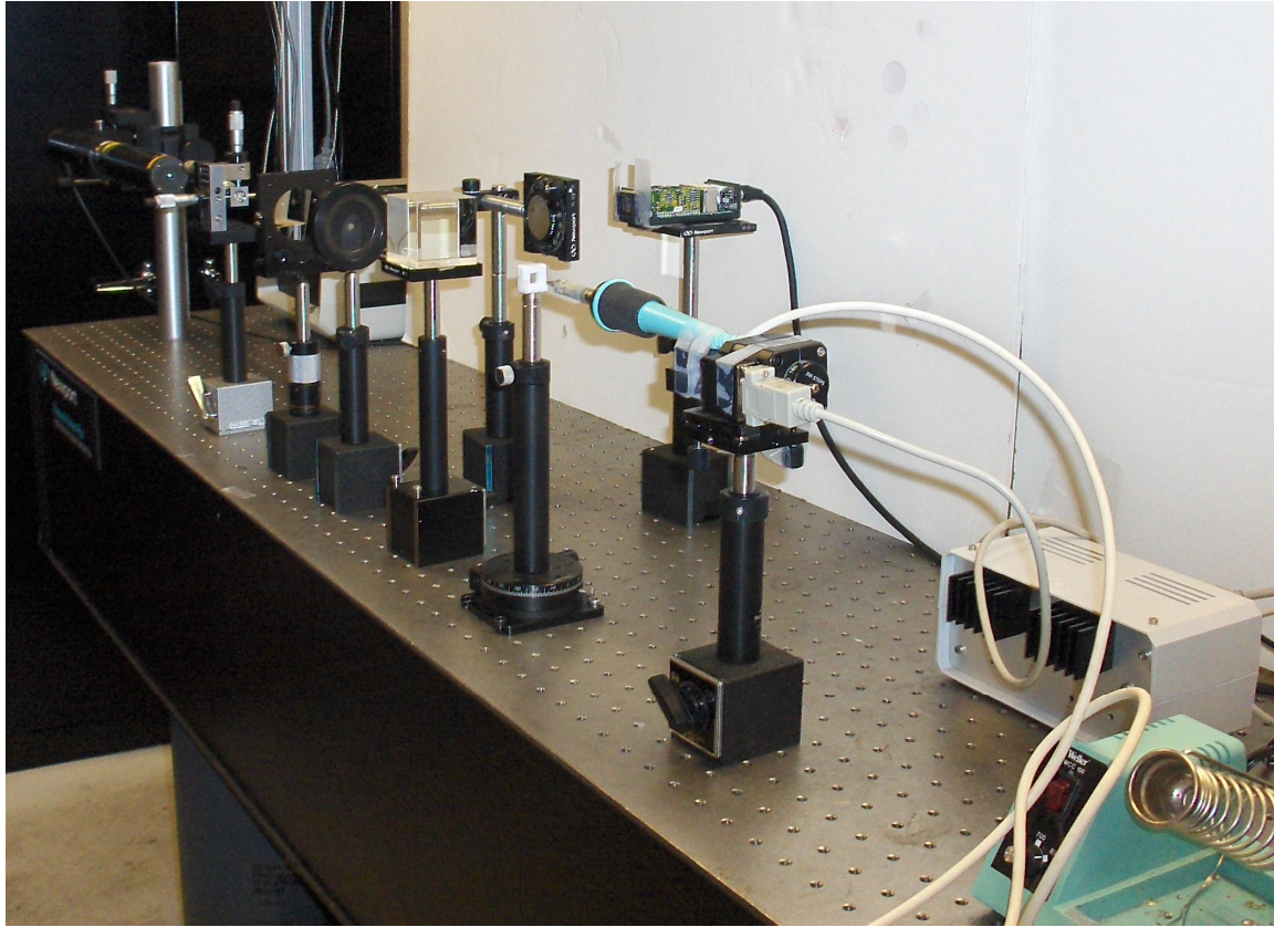
Fig. 2. Experimental arrangement used in the lab to measure the temporal response of the SiC chip to an applied thermal step function.
