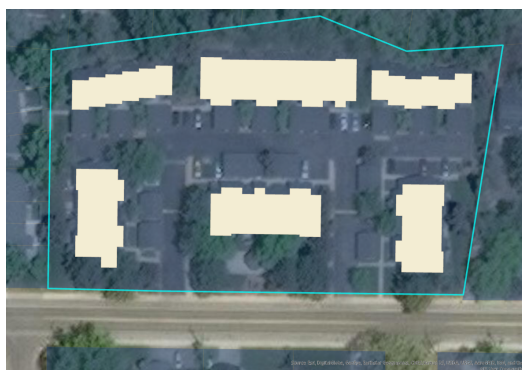
(a) Blue line represents the parcel data, which is the calculated acreage. Capacity calculation requires the building footprints individually, indicated in beige.
