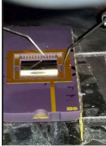
Figure 4.7 Testing of the Package Part on the Micro-Manipulator Probe Station
