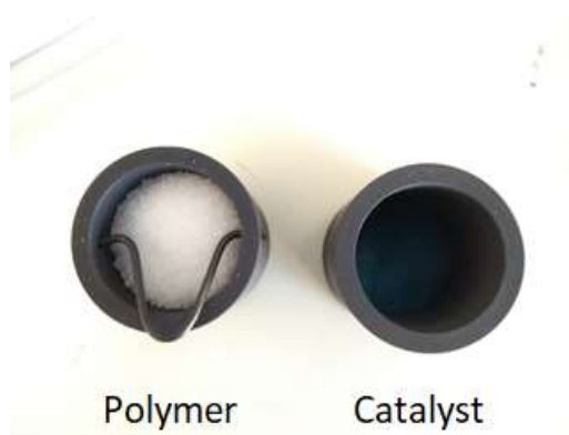
Figure 23: Crucibles containing polymer (low-density polyethylene) and catalyst (20% Ni/Al).
