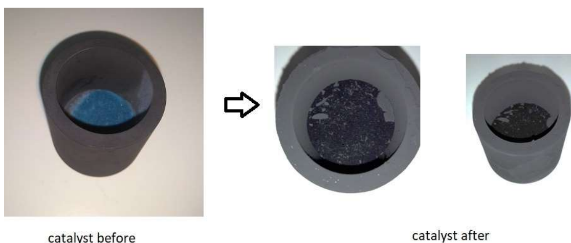
Figure 24: Crucibles containing carbon structures by chemical vapor deposition.
