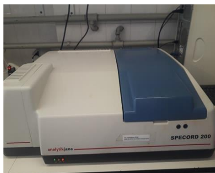
Figure 3. SPECORD®200 spectrophotometer used in this work
