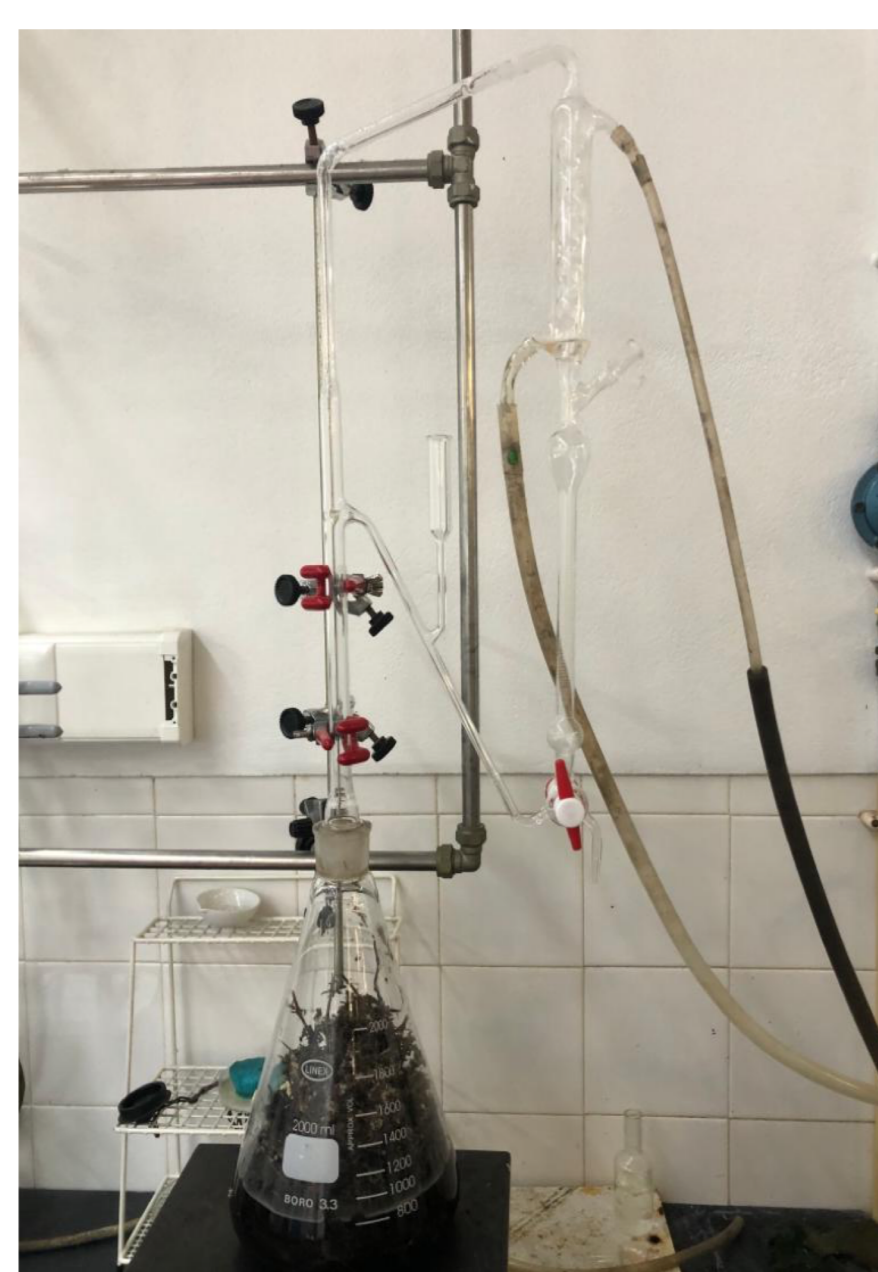
Figure 1) Extraction of Salvia elegans EO in Clevenger apparatus.
