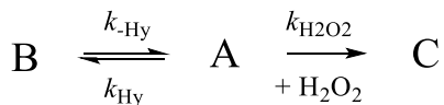
Scheme 1: Model used to fit the reaction between sodium pyruvate and H 2 O 2
