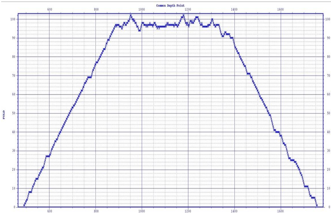
Figure 2.1 CMP fold coverage for the binned dataset. The maximum obtained CMP fold (top of the plot) is 105.
