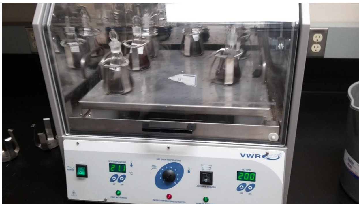
Picture of arranged flasks containing samples of gold solution and bioadsorbent in a shaker
