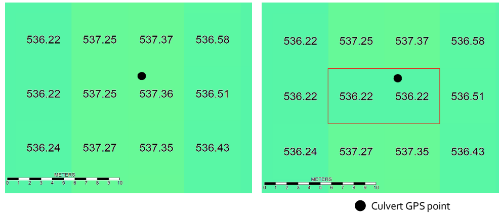
Figure 2.3 Example of a culvert burning process in open source GIS software SAGA. The light green in both images represents a road network in the DEM, while the darker green on either side are waterbodies. The point on the road is a given culvert location. The DEM grids corresponding to the culvert points were changed to the lowest elevation within the same areas (left image)
