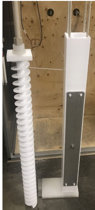
Figure 4.1: Vertically oriented parallel plate through field type applicator and teflon composite augur system.
