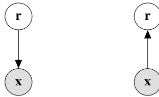
Fig. 2.2 The directed graphical model illustration of an autoencoder. The encoder (right) is the function \mathbf{g}_\phi(\mathbf{x}) \rightarrow \mathbf{r} parametrised by \phi (equation 2.14), which maps an input \mathbf{x} to its representation \mathbf{r} . The decoder (left) is the function \mathbf{f}_\theta(\mathbf{r}) \rightarrow \hat{\mathbf{x}} parametrised by \theta (equation 2.15), which maps a representation \mathbf{r} back to a reconstruction of the input \hat{\mathbf{x}} .
