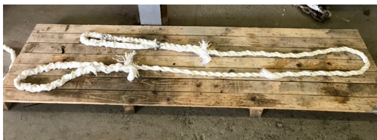
Figure 11. One broken strand near end of eye splice (Test 02 at DMaC), representative of the dominant failure mode.
