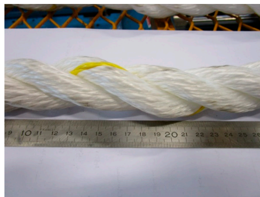
Figure 1. Twisted rope construction of the hybrid polyester-polyolefin rope.
