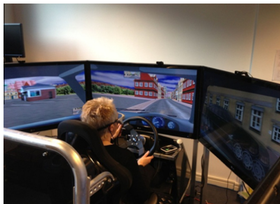
Fig. 1. Fixed-based ST Software Jentig50 driving simulator.
