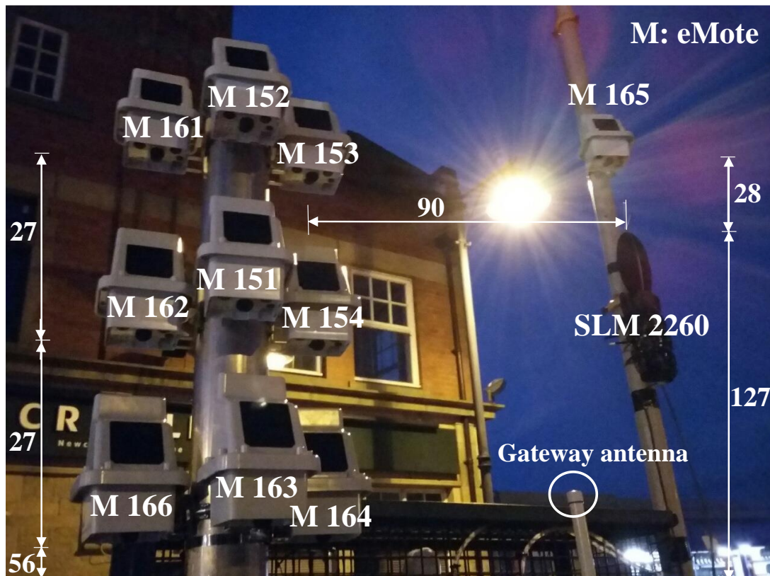
Figure 6 Experimental layout showing co-location of precision system and eMote units at the Cradlewell AURN cabin (distances shown in cm)
