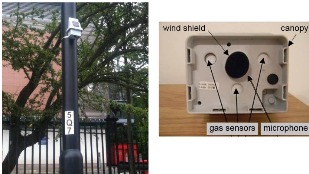
Figure 2 eMote mounted on a lamppost (left) and close up of sensor payload (right) [22]
