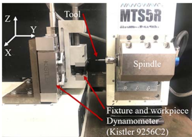
Fig. 4 Machine setup with cutting force dynamometer
