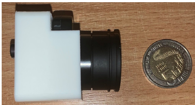
Figure 2. FLIR Boson In a 3D printed case next to a coin for scale, the camera weighs around 7.5 grams.
