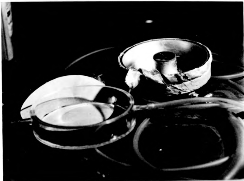
Plate P.7 The Mark IV annular channel with the heater coil insulation partly opened.
