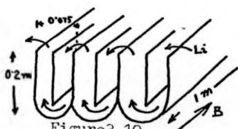
Figure 2.10 The slim channel design of the Wisconsin device.
