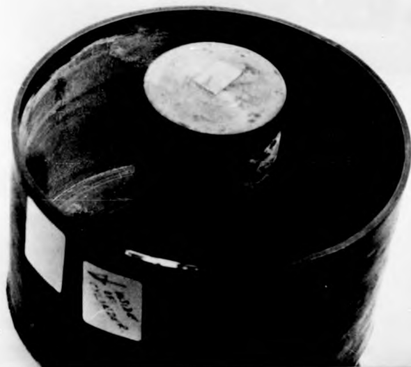
Plate P.3 The etch marks on the Mark I annular channel inner surface at the outer periphery.
